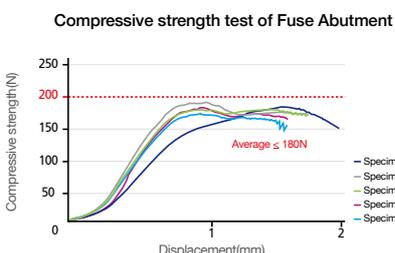
Performed compressive strength test to evaluate the yield strength for Fuse Abutment using universal testing machine
