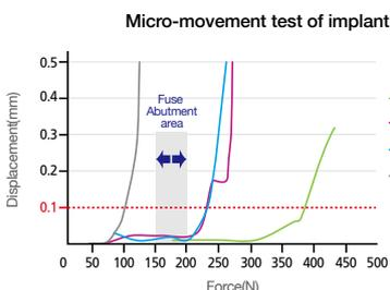
Performed compressive strength test to evaluate the micro movement for bone density using universal testing machine
