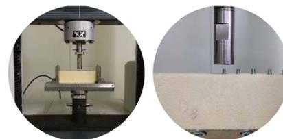
From this experiment, we could developed a special temporary abutment which has lower fracture threshold of less than 200 N (20.4 kgf). It was named as Fuse Abutment. Also it has an anatomic profiles to make temporary prosthetics more esthetic.
